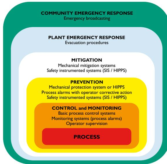
The IEC 61508 mainly focuses on Electrical/Electronic/Programmable Safety-related systems. However it also provides a framework for safety-related systems based on other technologies including mechanical systems. The IEC 61511 was introduced by the IEC specifically for designers, integrators and users of safety instrumented systems and covers the other parts of the safety loop (initiators and final elements) in greater in detail.
