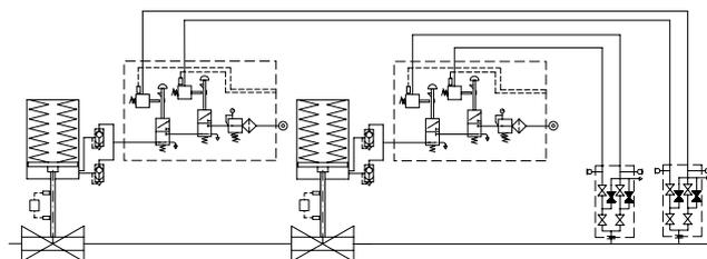
Example of a HIPPS consisting of 2 final elements each having two mechanical initiators, SIL 4 is obtained. Testing can be done via the high integrity manifold block with key interlock system.
