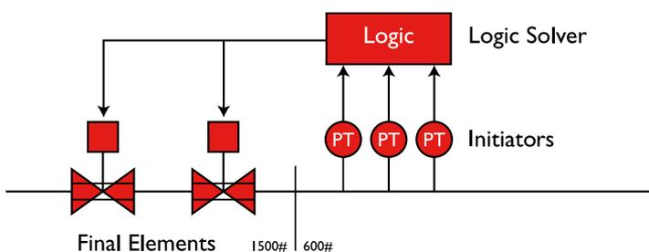
A typical HIPPS safety loop consisting of 2oo3 initiators (Pressure Transmitters), a logic solver and 2 final elements being valve and actuator.
